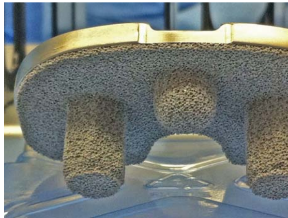
The underside of a cementless tibial component used for Dr. Fricka's study illustrates the porous trabecular metal surface that has a structure similar to human trabecular bone.
